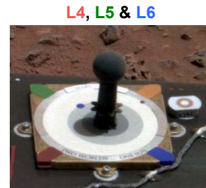
Figure 2. Color Chart Reflectivity Measured by NASA Under Martian Illumination
