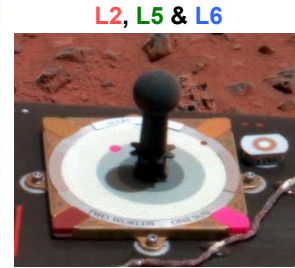
Figure 3. MER Calibration Targets Viewed Under Terrestrial and Martian Illumination
